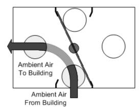
Figure 6 - Recirculation Mode without Compressor.
