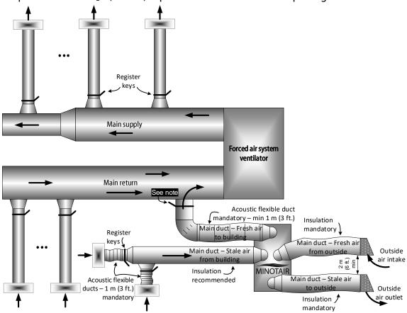
Figure 10 - Connection to a forced air ventilation system - Extraction at the source.
