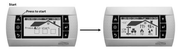
Figure 29 – To turn on the MINOTAIR, press ▲.
