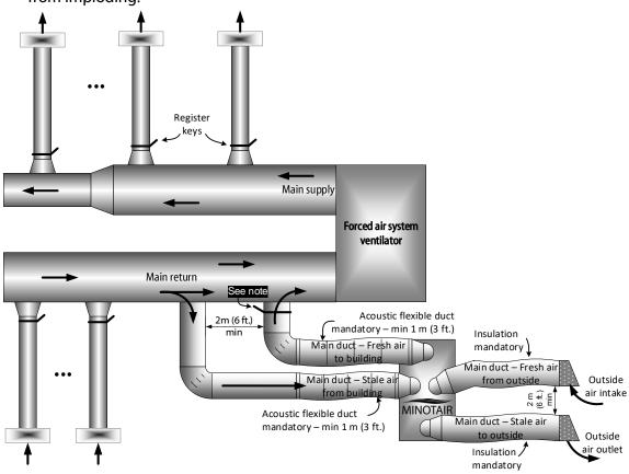
Figure 9 - Connection to a forced air ventilation system - Simplified method.
