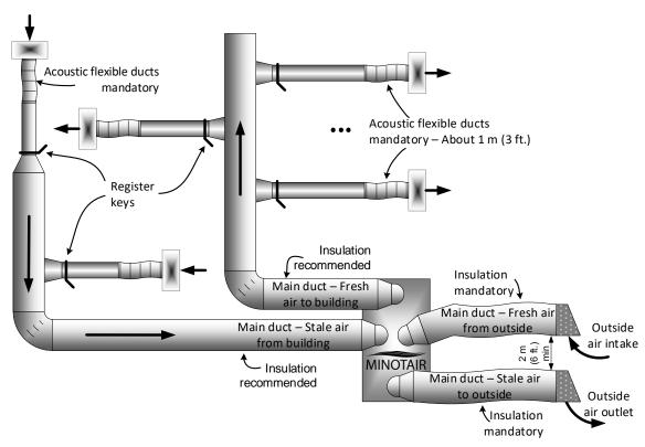
Figure 11 - Connection to an independent system of ventilation ducts.
