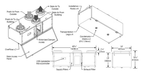
Figure 3 - External overview of the device.
