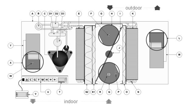
Figure 2 - MINOTAIR assembly and components (image for conceptual purposes only).
