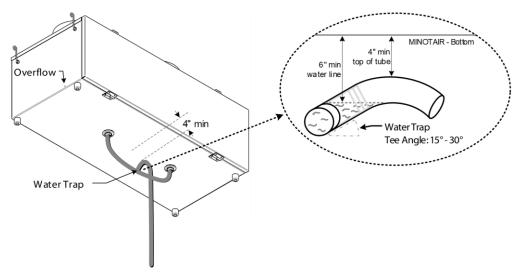
Figure 15 - Position the Tee fitting to form a water trap between the two drains.
