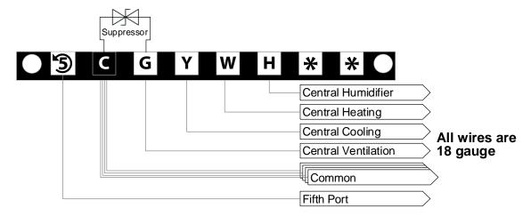
Figure 16 - Connection to a forced air ventilator and other auxiliary devices.
