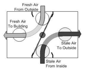
Figure 4 - Air Exchanger Mode (Ventilation).
