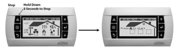
Figure 30 – To turn off the MINOTAIR, hold down  $\triangle$  for 3 seconds.
