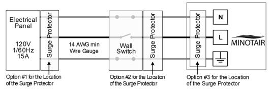
Figure 24 - Connecting the device.
