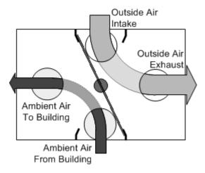
Figure 5 - Heat Pump Mode (Recirculation with Compressor).
