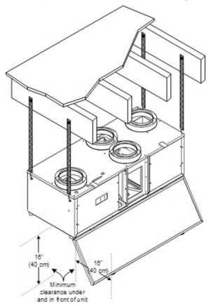
Figure 14 - Mounting the MINOTAIR using the floor joists.
