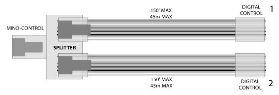
Figure 22 - Cable configuration for two wallmount digital controls
